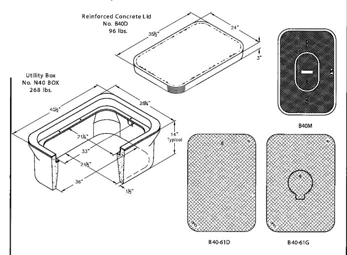
A high density reinforced concrete box with non-settling shoulders positioned to maintain grade and facilitate back filling. Approximate dimensions and weight shown.
